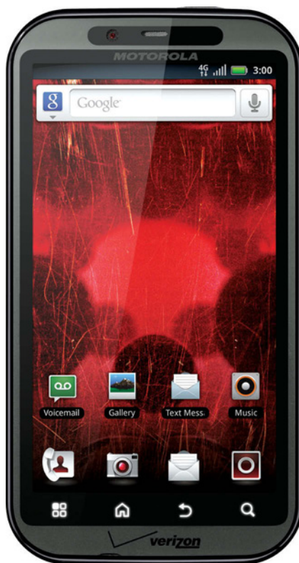
Smart phones such as the Motorola Droid Bionic use the tiny but powerful Tegra 2 chip for general phone operations and graphical display.
