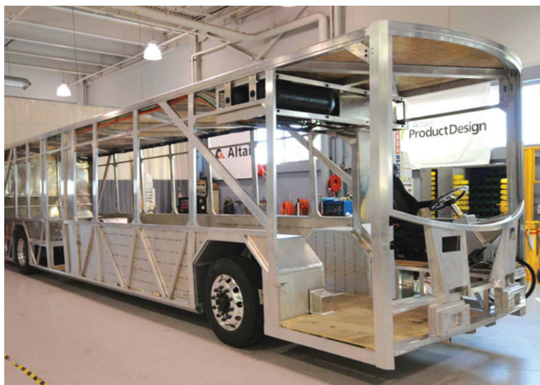
THE LCO-140H has a lightweight aluminum construction. Structural support was placed according to analysis results.
