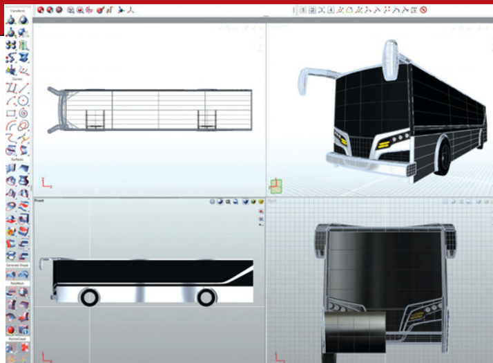
SOLIDTHINKING was used to quickly evaluate multiple design themes for the transit bus.
